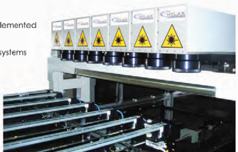
Inside of a 7-Heads ScanVision™ Laser FPD Marking Machine
