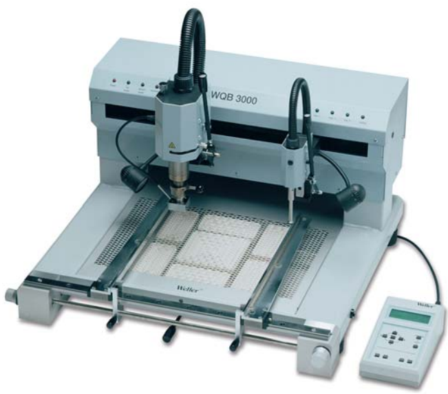
WQB 3000 BGA/SMT rework system for component placement with templates
