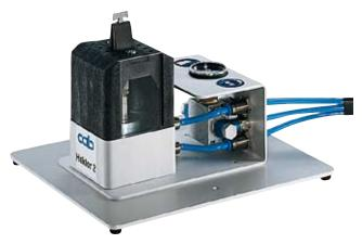
Hektor separates milled PCBs carefully and fast. The offcut material is removed smoothly and precisely. The matrix consists of two parts. This ensures easy and cost-saving change of the blades. Compressed air is used for the separation process. The operating pressure can be set on the machine. When the foot switch is pressed, the off-cut is punched out. The off-cuts are collected in the collecting box. When the gate is opened the waste material can be extracted.
