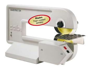
MAESTRO 2 separates small amount and prototype series of PCBs fast and economically. The compact and stable aluminum frame requires only a minimum of space.
