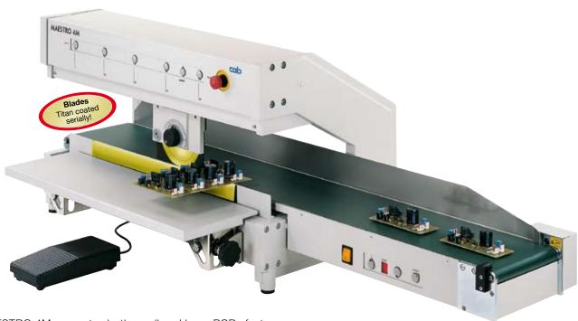
MAESTRO 4M separates both small and large PCBs fast and economically. To optimize operation, the separation length can be programmed with the control keys.
