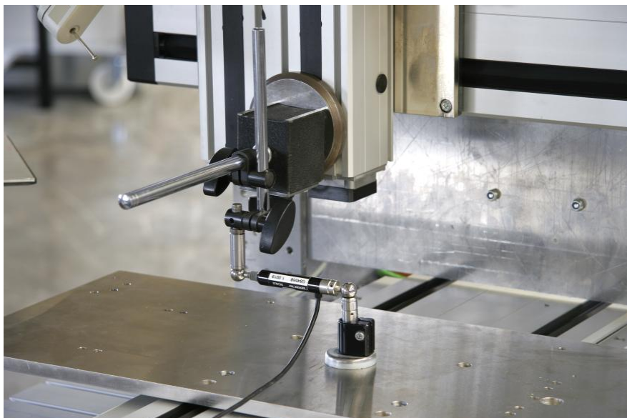
picture: circular form measure with Renishaw QC10
