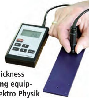
Layer thickness measuring equipment Elektro Physik
