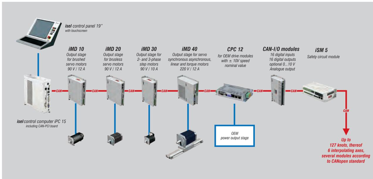
With consequent use of the CiA's (CAN in automation) **CANopen** standards, isel Germany delivers a high quality PC-based **CAN-CNC controller** for intelligent positioning/drive units and I/O modules.
