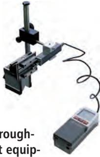
Surface roughness test equipment Mitutoyo
