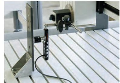
Renishaw's QC 10 system is used to check machine accuracy. This system determines the relative accuracy of the axes of a machine tool. Circular dimensions are controlled using a simple CNC program. The form of the circles generated gives information any potential faults present.
