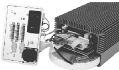
Applikation with toroidal core transformer, printed circuit board and front plate
